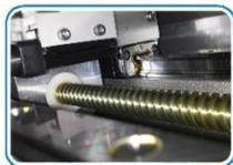
Closed-loop servo drives, linear guides & ballscrews provide stability & smooth accurate motion
