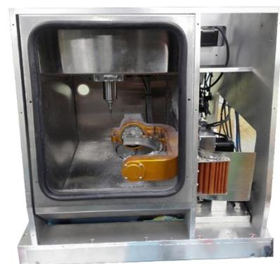
*Figure 1: Aluminum frame while offering strength and rigidity provide less vibration dampening than cast machine frames.*
