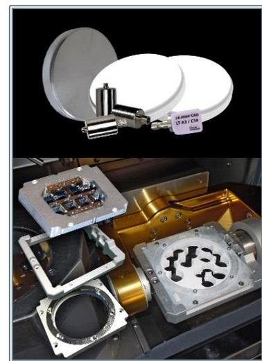
Figure 5. Versamill 5X-200 Universal Fixture offering complete stability and versatility. Notice fully-supported fixture held on both ends with precision cartridge inserts to enable quick change-over to different rough stock forms.
