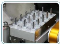
15-position ATC w/auto length compensation & breakage detection.
