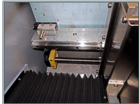
*Figure 6. Internal view of the versamill 5X-200 showing use of precision ballscrews w/anti-backlash nut, large way-surface with linear guide and protective coverings. All elements found in "large-format" high-speed industrial machines but less common in a DMC.*
